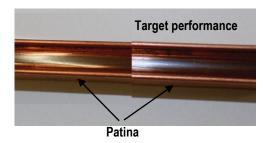
c) Cleaned copper rail (copper coloured rail with scrub marks)
