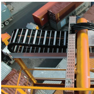
Conductix-Wampfler plastic chain with aluminium strays on a port crane
